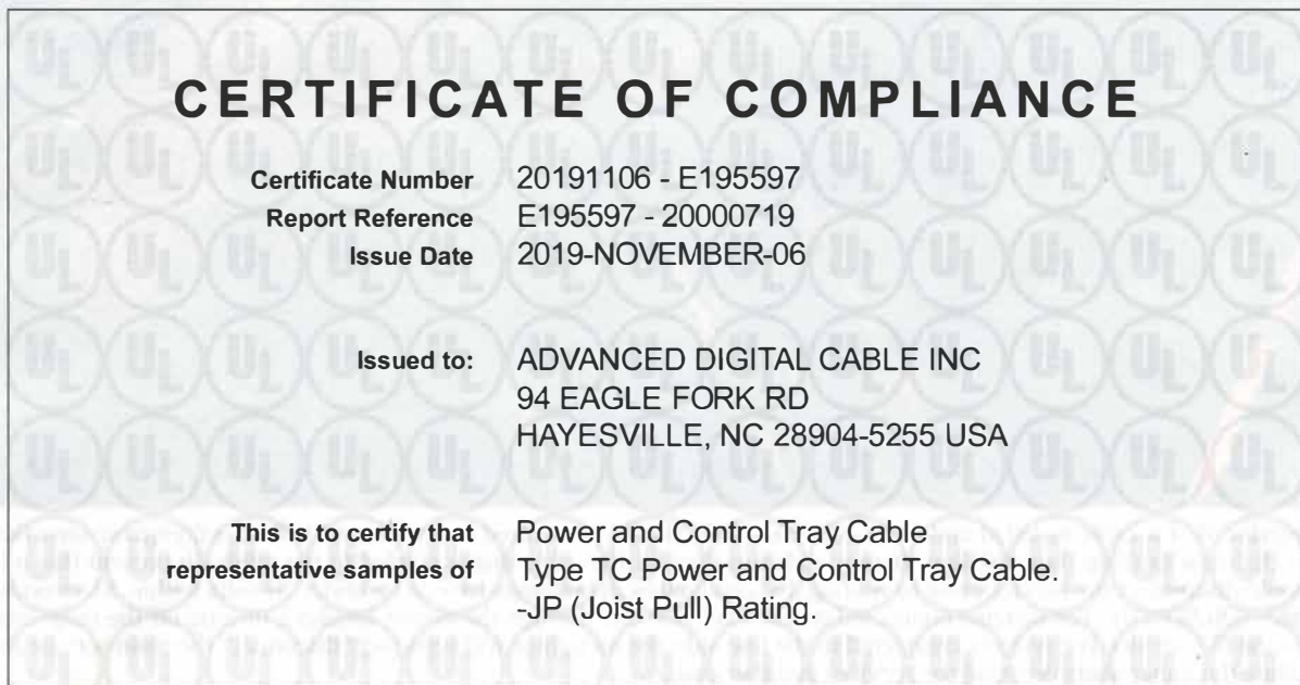
Photo 2. Example of a UL Joist Pull Listing for TC-ER cable
